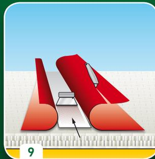
9 Cut the artificial grass to size, lay down seam tape between the joins and apply an even layer of adhesive.
