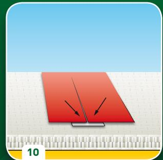
10 Press the artificial grass onto the adhesive and leave it to dry properly.
