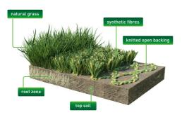
Avalon Urban Hybrid is a sturdy knitted artificial grass mat topped with fibers in different pile heights. The mat has wide openings in the form of a honeycomb structure. These wide openings allow the natural grass to grow. This unique knitted honeycomb structure provides reinforcement to the root zone of the natural grass. In addition, the artificial grass fibers protect the blades of the natural grass from wear and tear.
