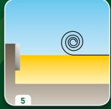
Roll out the geotextile on the sand bed to protect against weeds. Overlap individual rolls by 5-10 cm.
