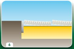
Lay down the PE foam mats (thickness depends on HIC certification).
