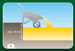
Excavate at least 15 cm of earth and lay down a bed of sand.
