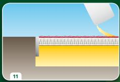
Make a small slice at the bottom of the sand bag and fill the artificial grass with silica sand using 5 kg/m2 (grain size: 0.25 - 1.25 mm).
