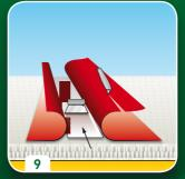
Cut the artificial grass to size, lay down seam tape between the joins and apply an even layer of adhesive.
